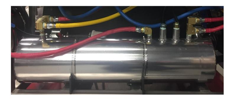
**Exhaust Heat Exchanger,** is a S.S. tubular heat exchanger, which captures the hot engine exhaust to boost the pre-heat water from the coolant heat exchangers to a consistent high heat. This heat exchanger is ceramic coated to keep the heat in the exchanger and to reduce the radiant heat in the vehicle.
