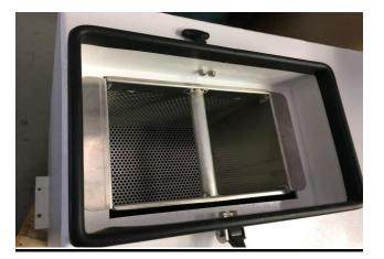
Waste Tank Blower Inlet Filters On the inside of the waste tank are two filters. These filters prevent any particles from entering the vacuum blower. It is very important to remove and clean these filters on a weekly basis, or more if needed. Before reinstalling the filters apply some lubricant / grease on the thread of the filters and only hand tighten the filters, this makes it easier to remove them the next time. Blower Filters Part Number 560-205.
